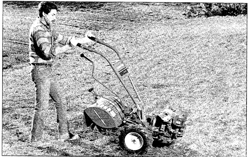
Photo 4-9: To turn the tiller around most easily, lift up handlebars to find “balance” point between engine and tines, then push against handlebars in the direction of the turn while the powered wheels do the hard work.
